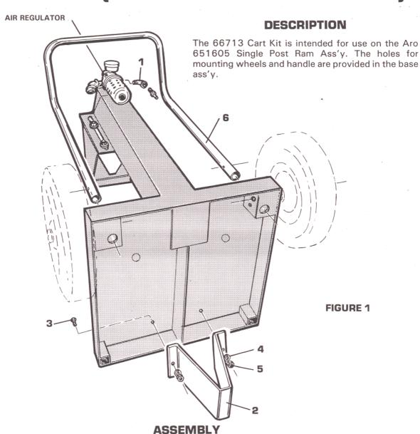
Remove inlet connector from air regulator and install 1 street elbow. Reinstall inlet connector into 1.
